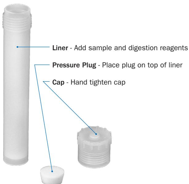
**Figure 1:** MARSXpress 3-Part Vessel
